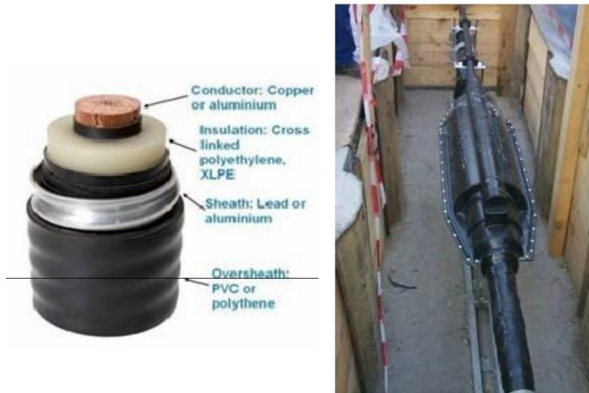
Figure C.4 – Cable Cross-Section and Joint
